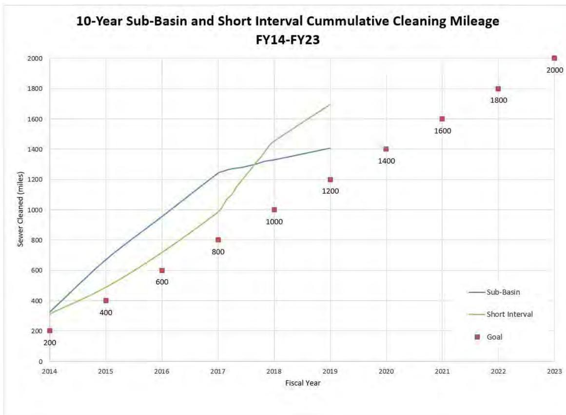
Figure 5 Small Diameter Sewer Cleaned vs. Ten-Year Goal
