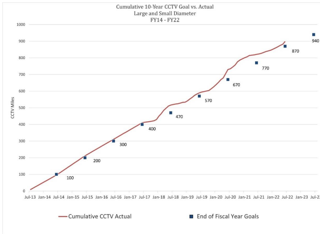
Figure 3 Small & Large Diameter Sewer CCTVed vs. Ten-Year Goal
