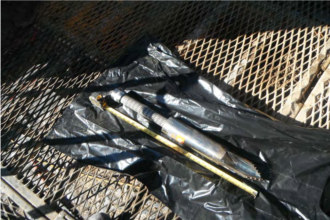
No. 12 – Push-ahead ground water sampler.
