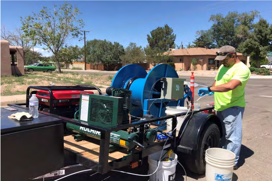
No. 32 – Photograph of the low flow sampling trailer and flow rate being measured.
