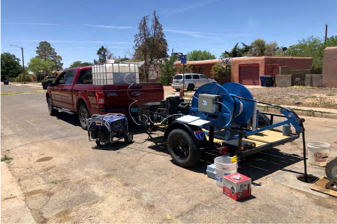
No. 31 – Photograph of the low flow sampling set up using a trailer mounted Bennett Pump.
