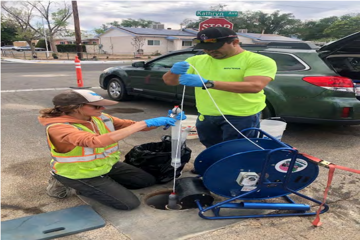
No. 29 – Photograph of the PDBs being pulled up for sampling.
