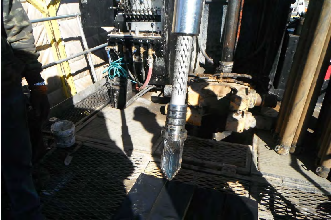
No. 13 – Push-ahead ground water sampler.
