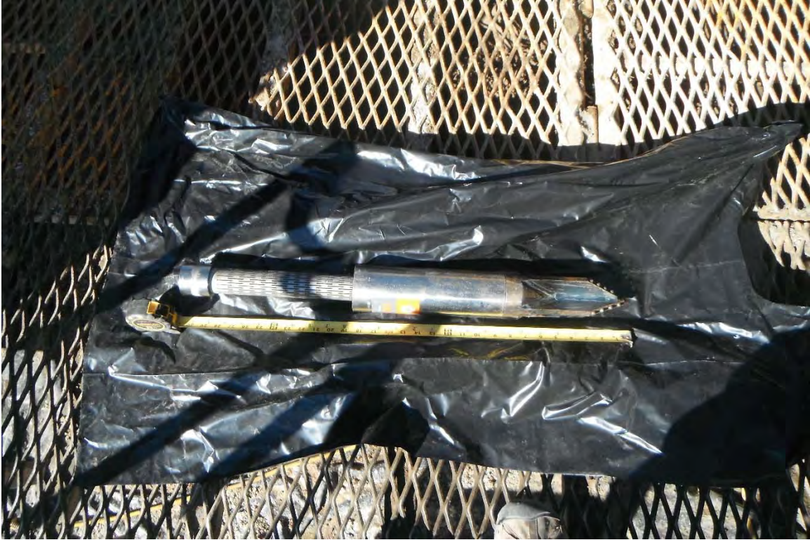
No. 11 – Push-ahead ground water sampler.
