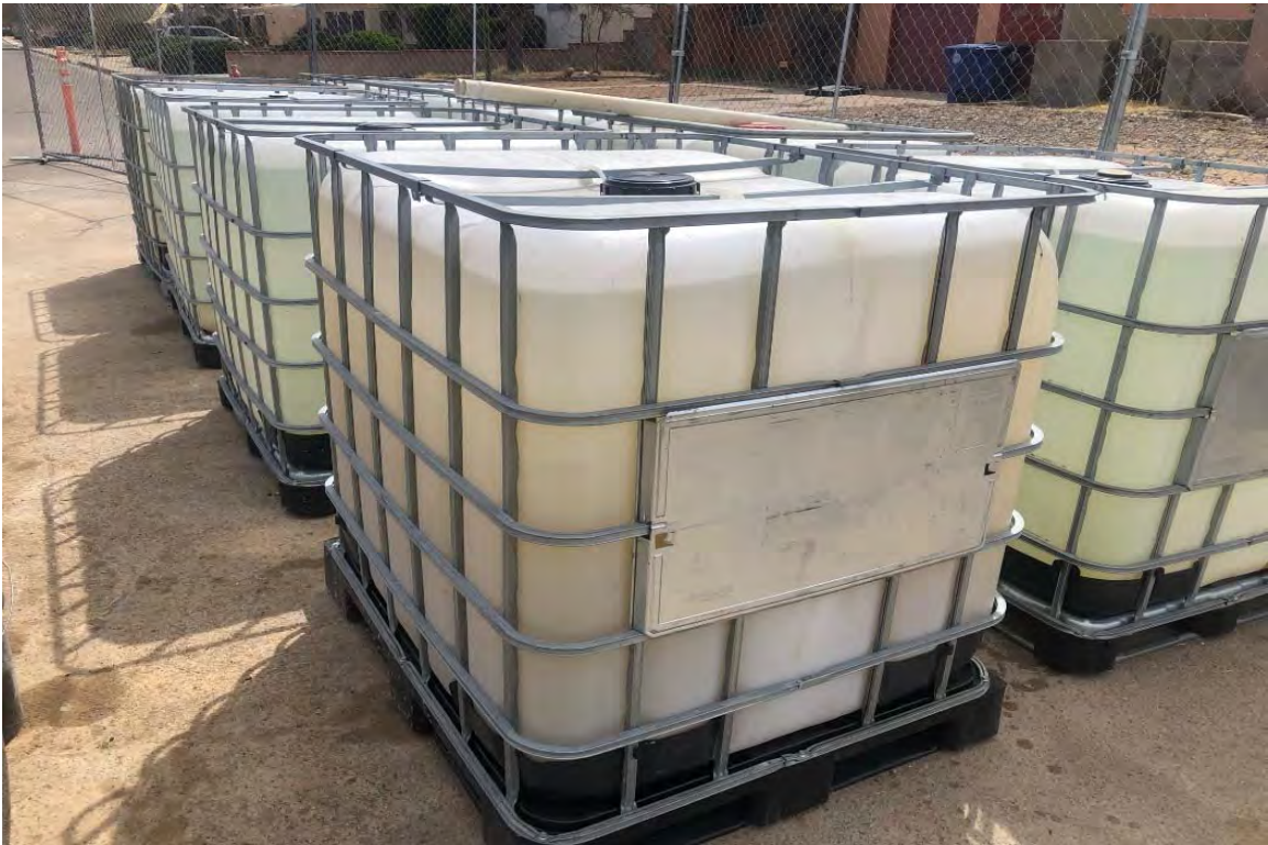
No. 28 – Photograph of the 275-gallon totes that the development water was stored in on-site.
