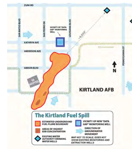
ABOVE Map showing extent of the Kirtland underground fuel spill and location of the new data gap monitoring well.
