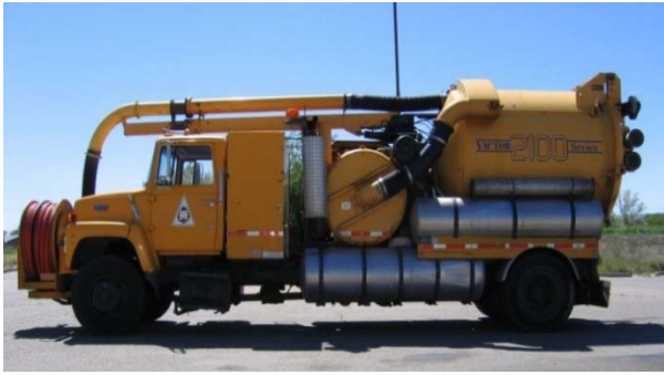
Sewer Cleaning Truck (Vactor)
